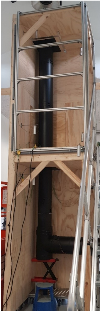
Photo 1: Chimney installed in thermal test rig
